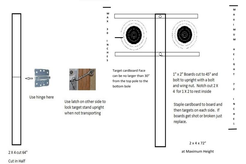
This is a recommended target for people carrying their target in their truck or car because the hinge allows you to fold it in half.
